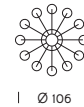
1380/12 con gocce - with drops 1382/12 senza gocce - without drops 12 x MAX 42W E14 (E14)
