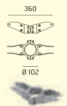
222 DOUBLE BRACKET 180mm FOR POLE Ø 102mm
