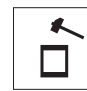
Protection against impact. IK 05 - 0,70 joule for Pi 50x50 IK 07 - 2,00 joule for Pi 70x70
