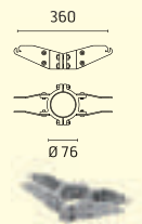
230 DOUBLE BRACKET 180mm FOR POLE Ø 76mm
