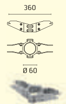
226 DOUBLE BRACKET 180mm FOR POLE Ø 60mm
